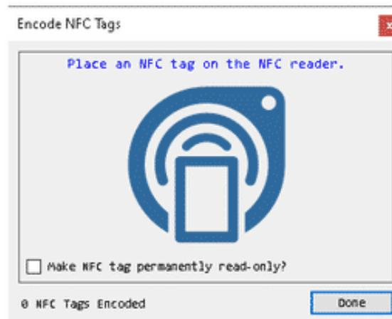
10. Wait until the software confirms that the NFC tag is properly encoded.
