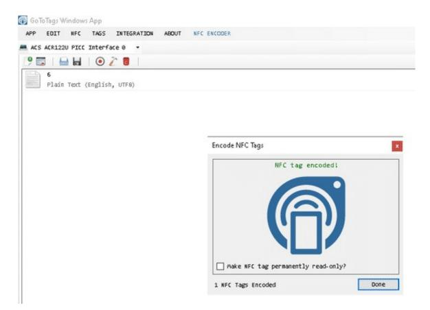
Your NFC tag is now ready for reading by the FISHGUN. For encoding a new blank NFC tag with the same number, proceed to step 9. Otherwise, you only need to erase the data entered in the box using the "Clear all records" icon.
