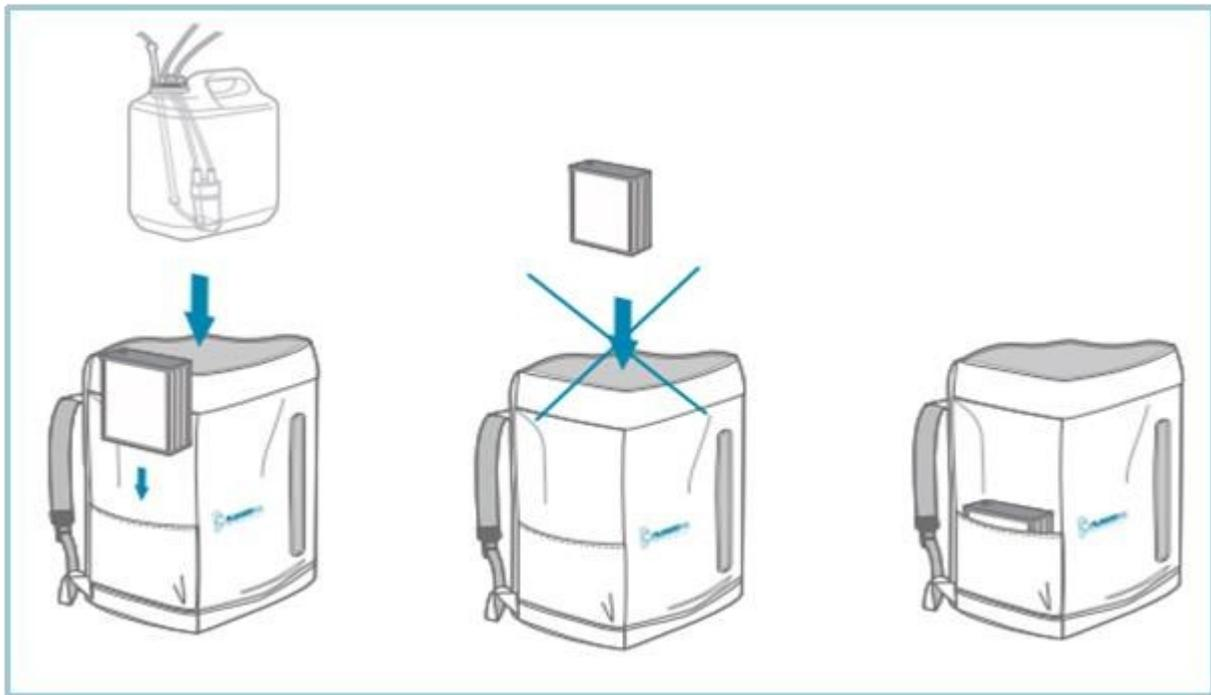
If the liquid touches the controller case, remove the case and dry it with a cloth. The maximum capacity of the tank is 5 liters, moreover, we advise not to fill above 4.5 liters in order to avoid any overflow during transport while feeding. The 5L tank is a suggestion, you are free to use another tank (with a tank capacity bigger or equal to 0.5L) to hold the liquid feed.
